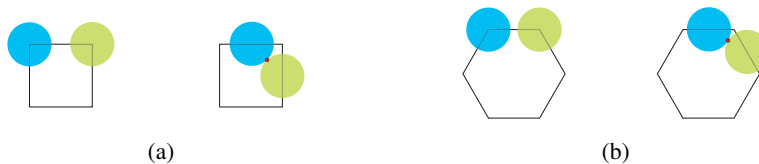
Fig. 3. Minimum distance between robots. To ensure no collision when executing a discrete plan, the distance between two lattice nodes must be 4/\sqrt{2} + \epsilon for square tilings (a) and 4/\sqrt{3} + \epsilon for hexagonal tilings (b). At exactly 4/\sqrt{2} (resp. 4/\sqrt{3} ) the robots will touch when reaching the midpoint of the edge. The contact point is shown as a red dot in both figures.
